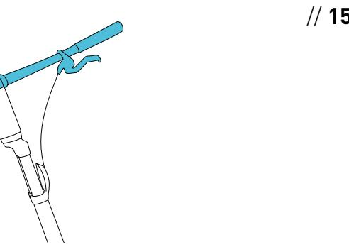
untighten screws on stem/fork connection and turn handle bar 90° clock-wise.
