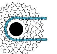
Chain on smallest sprocket
