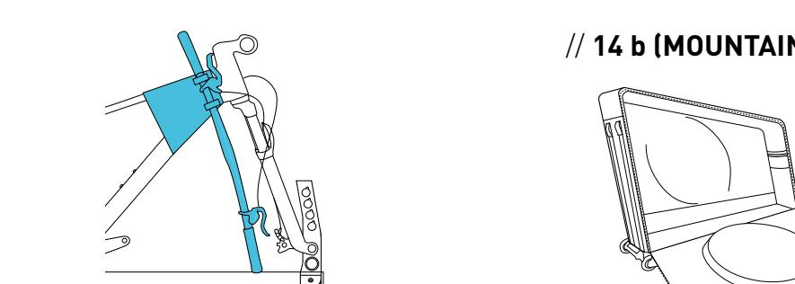
Remove handle bar and fix it on FRAME PAD
